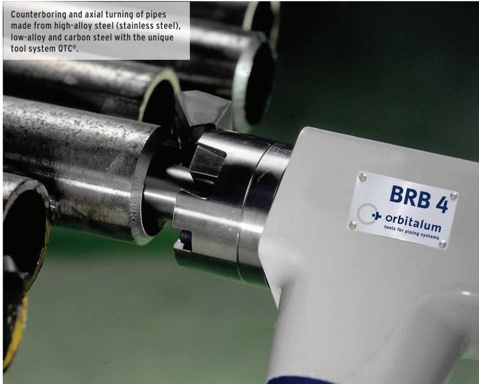
Counterboring and axial turning of pipes made from high-alloy steel (stainless steel), low-alloy and carbon steel with the unique tool system QTC®.
