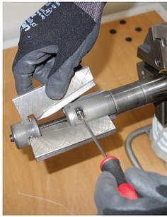
Fast adjustment of the pipe dimension
